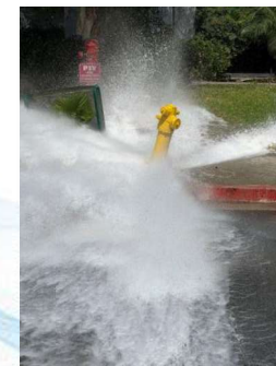
249 Paseo Tesoro Sheared Fire Hydrant
